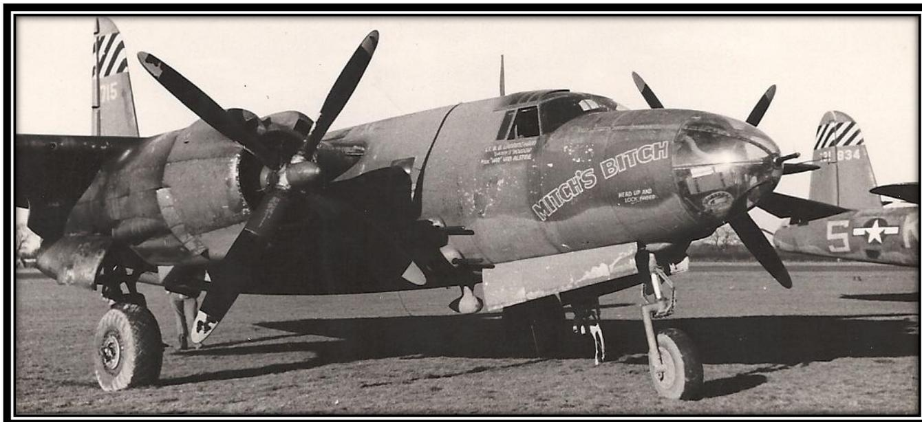
*Mitch’s Bitch*, a B-26B from the 387th Bomb Group’s 557th Bomb squadron. (serial number 41-31715, coded KS-P) Note the .50 caliber machine guns below and slightly behind the cockpit. Parked to its left is another 557th ship, *Alfy Snafu*. (serial number 41-31834, coded KS-S)
